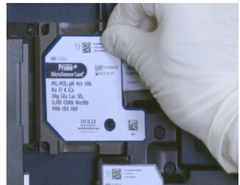
Figure 5.8 Remplacez la ABG MicroSensor Card
